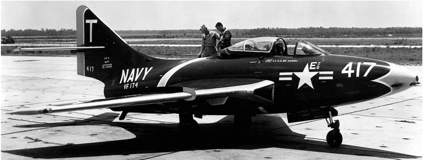
VF-174 F9F-6 127222 T417 pictured at NAS Cecil Field, on 15 June 1954. USN photo NMNA Coll. Note early F9F-6 configuration, lacking UHF homing antenna fairing beneath the nose and smaller (F9F-5 style) lower rudder. The trim and marking color is Light Yellow.
