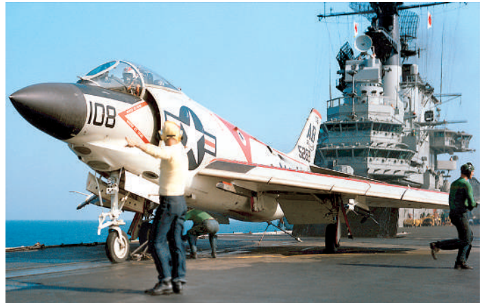
VF-14 F3H-2 145288 AB108 is hooked to the catapult with the bridle, on board CVA-42, on 20 June 1961. USN NA 428-KN-2352.
