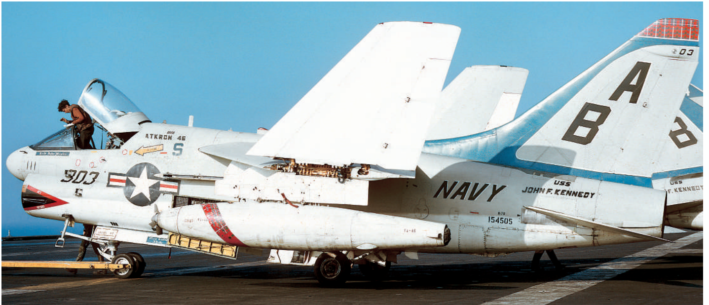
VA-46 tanker configured A-7B 154505 AB303 pictured aboard JFK, on 7 July 1973. Note the unusual ECM fairing fitted above the tail rudder. A. Gialanella photo.
