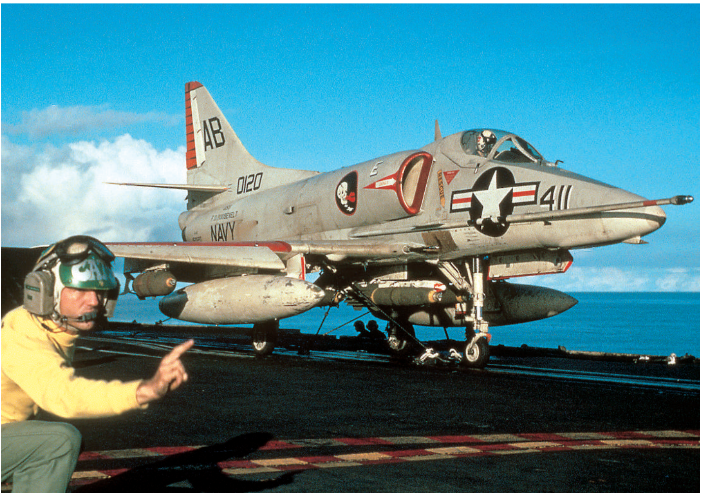
VA-12 A-4E Skyhawk 150120 AB411 loaded with M117 and Mk.82 bombs, while being readied and then launched for a strike mission, on 6 September 1966. USN NA 428-K-33067.
